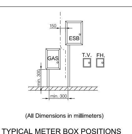
I CONFIRM THAT ALL GAS METER BOXES AND GAS SUPPLY PIPES SHALL BE INSTALLED IN ACCORDANCE WITH SK/701 AND ITS REQUIREMENTS.
